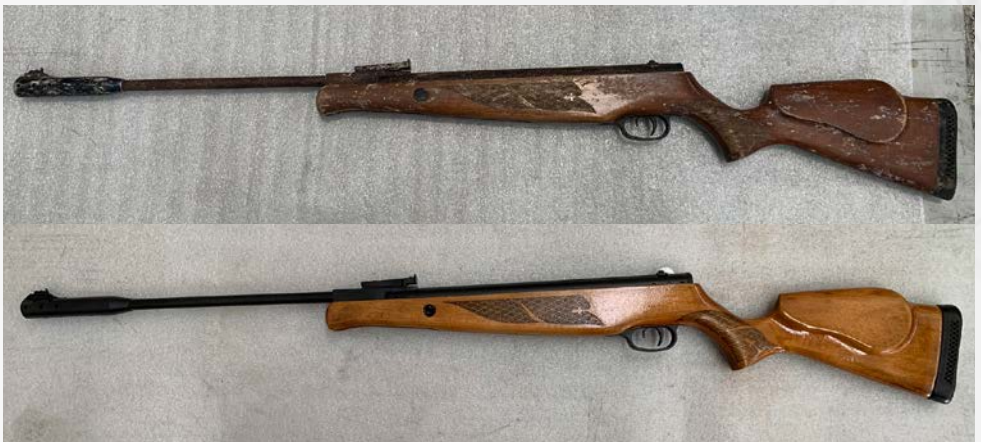
Example of restoration with TECNAN BLUE (Matt Black). The photo above, before the process, and the photo below shows the final result.
