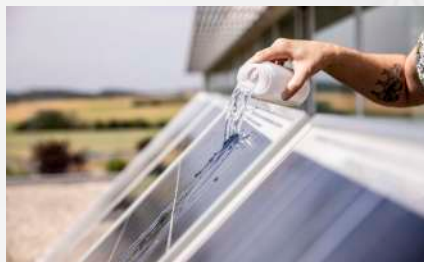
Hydrophilic effect on treated panel
