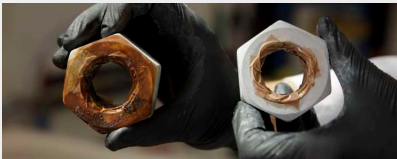
Example of two metal parts exposed to corrosion in a saline chamber, the one on the left without protection and the one on the right with Tecnadis Multicoat Anticorrosion
