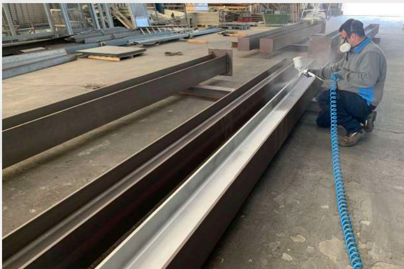
Example of application of Tecnadis Multicoat Anticorrosion (Primer) on a slightly oxidised surface
