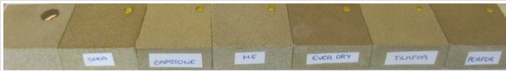
Untreated Sikaguard 917W Capstone ST200 Protect Guard MG Ultra Ever Dry Filafob TECNADIS PRS PERFORMANCE
