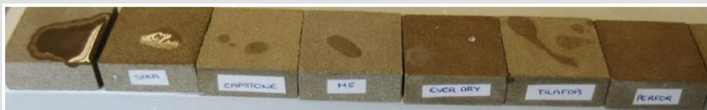
Untreated Sikaguard Capstone Protect Ultra Ever Filafob TECNADIS PRS 917W ST200 Guard MG dry PERFORMANCE
