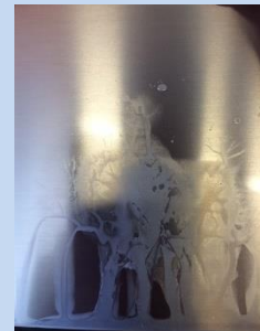
Not enough curing
