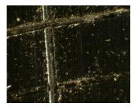
CONCLUSIONS: The cut edges are completely smooth; none of the corners
